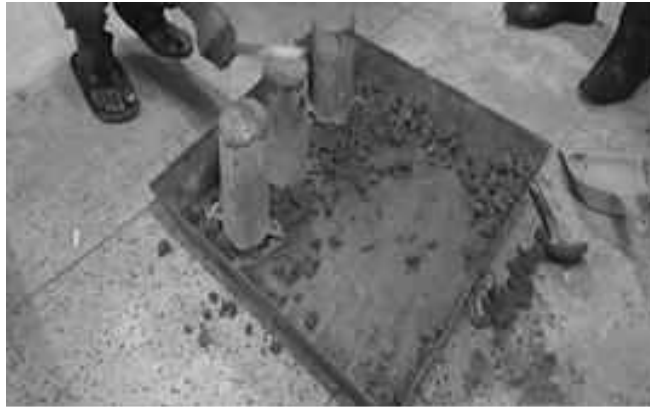
Figure 4: Making cylindrical specimen by using RA
