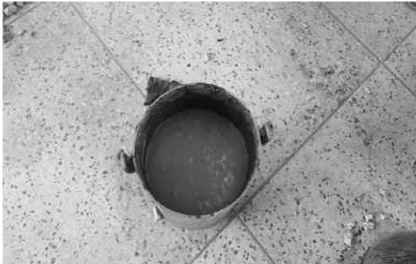
Figure 1: RA submerged in H_3PO_4 acid for removal of adhered mortar.
